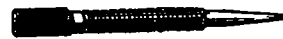
Nail set to drive nails into surface of the wood without leaving hammer marks
